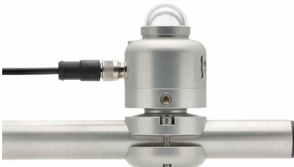
Figure 0.2 On the left SR05 digital second class pyranometer with bubble level and M12-A cable connector in its standard configuration (3 metre cable standard included); on the right SR05 with optional ball levelling, for easy mounting and levelling on (non-)horizontal surfaces (included mounting bolts not displayed)
