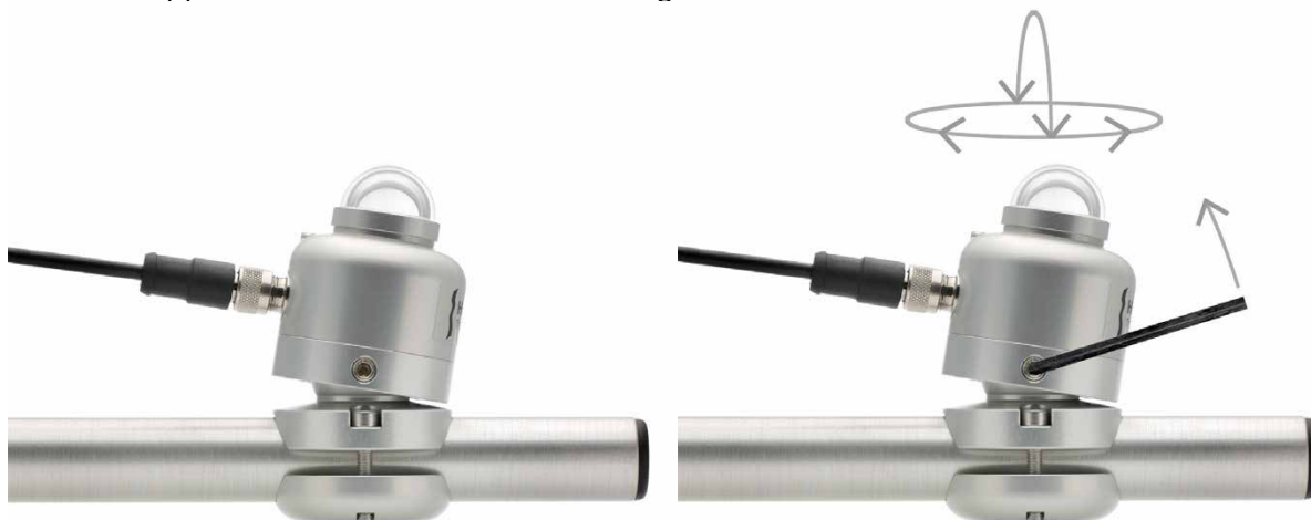
1) judge bubble level and cable orientation 2) loosen set screw to tilt and rotate SR05
