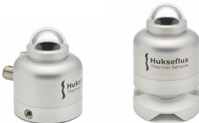
Figure 0.2 On the left SR05 digital second class pyranometer with bubble level and M12-A cable connector in its standard configuration (3 metre cable standard included); on the right SR05 with optional ball levelling, for easy mounting and levelling on (non-)horizontal surfaces (included mounting bolts not displayed)
