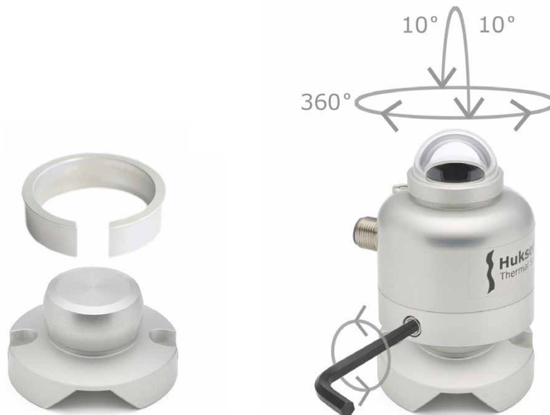
Figure 5.4.1 On the left SR05's ball levelling including shim (mounting bolts not displayed) and on the right SR05 placed on the ball levelling mount. Loosen the countersunk set screw on SR05's side to unlock, allowing placement of the ball head and SR05 levelling, and tighten it to lock the ball head mechanism. A 4 mm hex key is the only tool needed to place and remove the ball levelling and to allow and disallow levelling adjustment. The shim, included when ordering ball levelling, allows for smooth levelling and should be positioned properly in the centre of the bottom plate of SR05.
